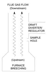
Figure 2-2. Installing the Probe
