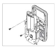
2. Loosen the two screws on the PCB to remove it from the front panel.
