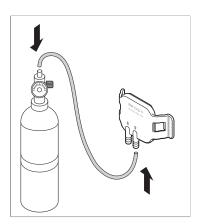
Connect a tube from a cylinder of calibration gas to the calibration cap's right spigot.
