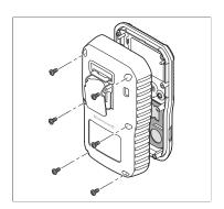
1. Loosen the six screws on the back of the detector to separate the front panel.
