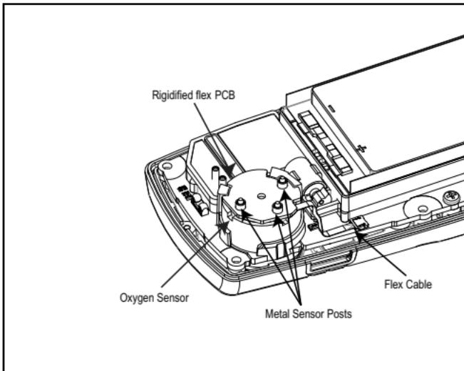
1. Gently remove the circular rigidified flex PCB atop the sensor from the metal sensor posts. Take care not to tear the flex cable.
