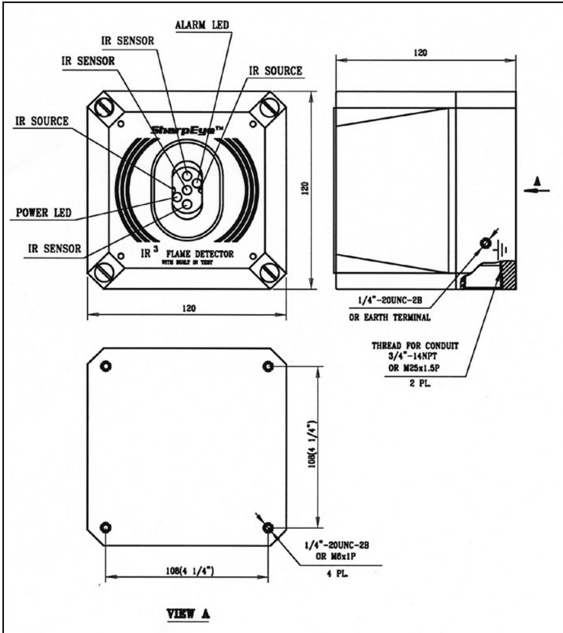
Figure 2: Flame Detector Assembly - Outline Drawing
