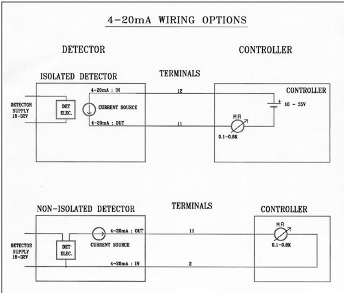
*Figure 16: 4-20mA wiring*
