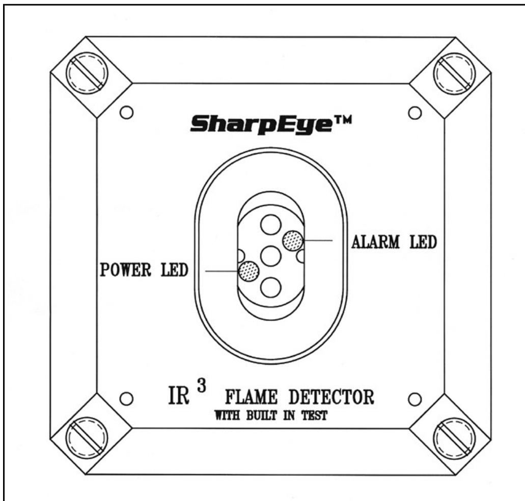
*Figure 4: Indication LEDs*
