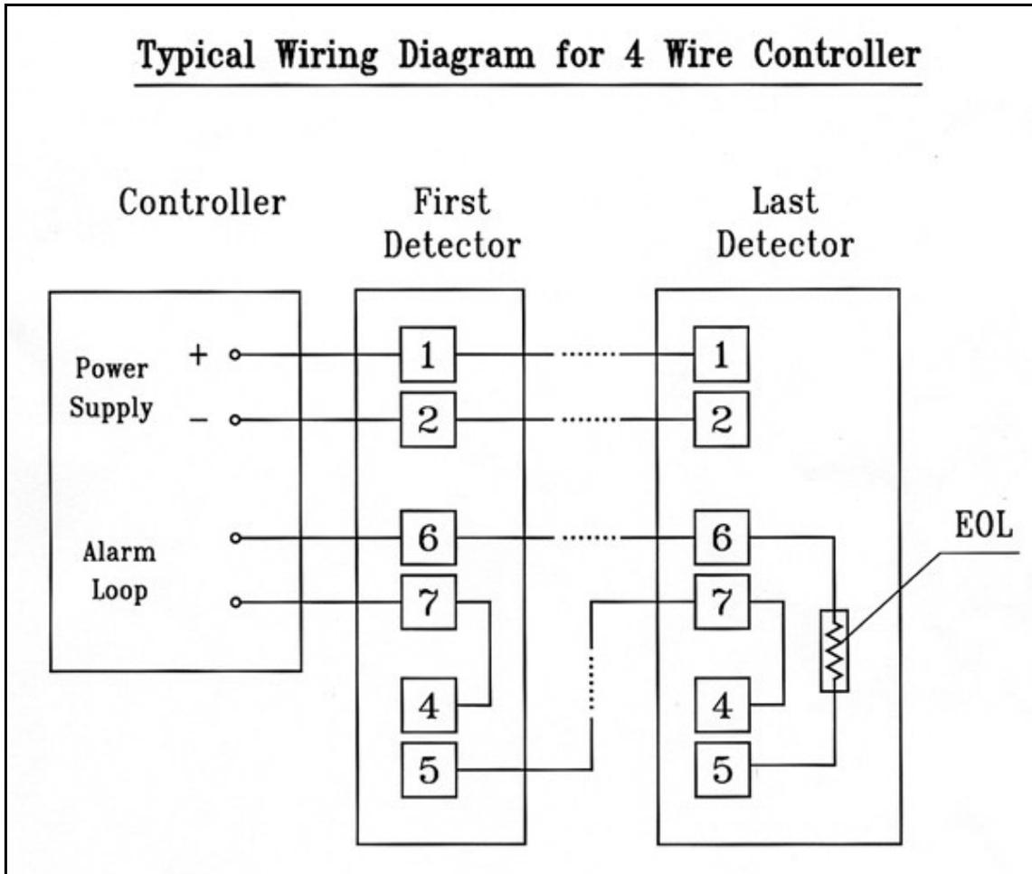
Figure 14: Typical wiring diagram for 4 wire controllers
