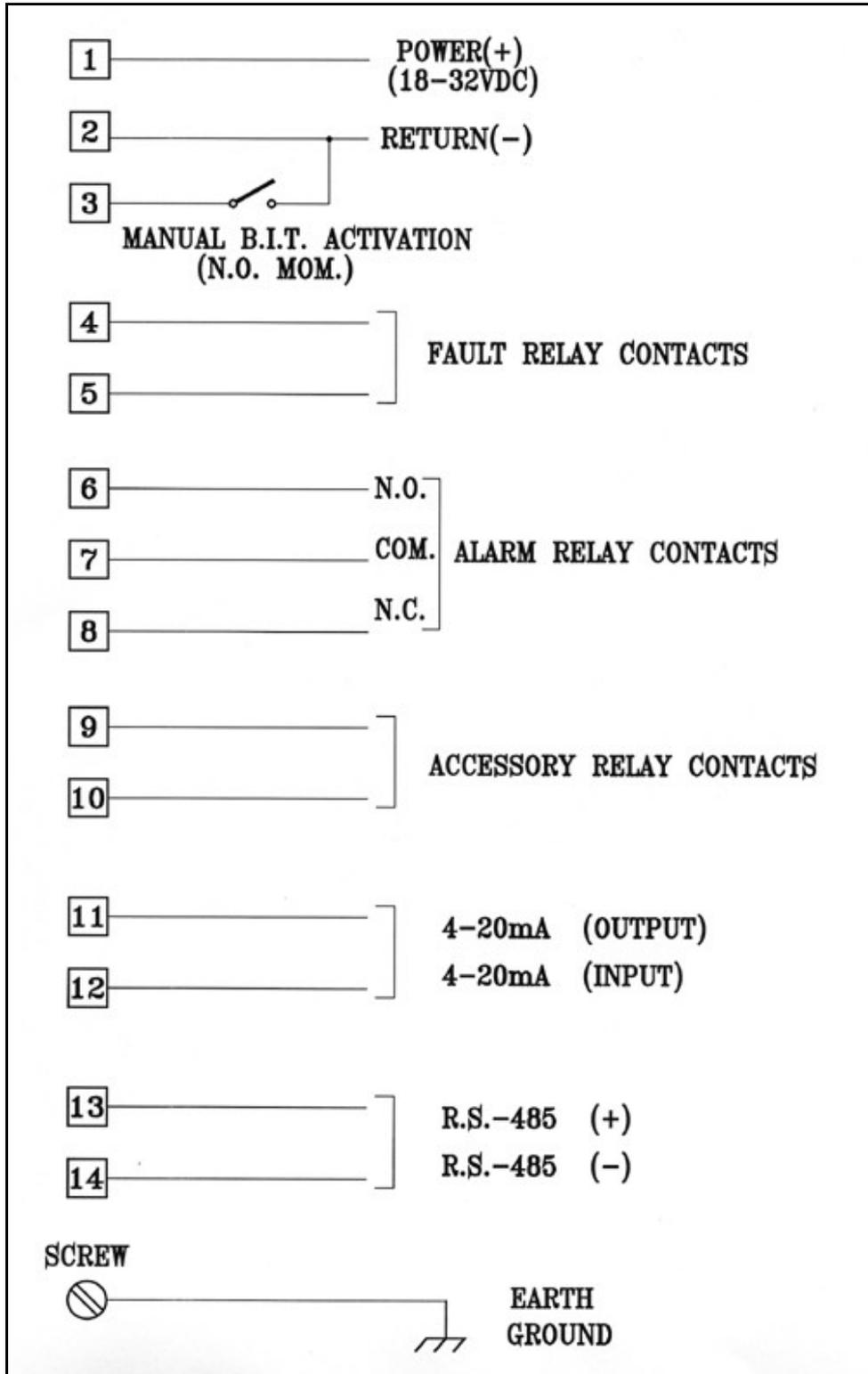
Figure 11: Flame Detector Assembly - Wiring Diagram
