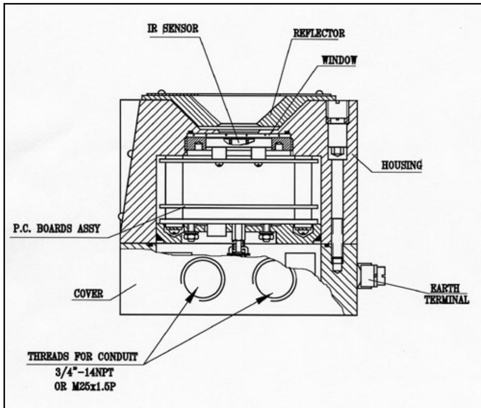
Figure 7: Flame Detector Assembly - Schematic Section
