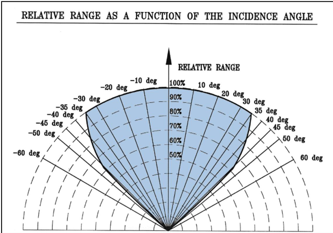
Figure 3: Horizontal and Vertical Fields of View
