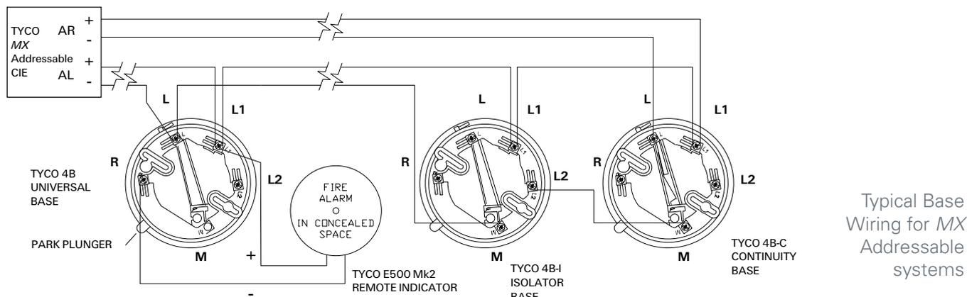
The MX CIE can be programmed to illuminate a Remote Indicator for detectors in alarm other than the detector base to which the Indicator is connected.
