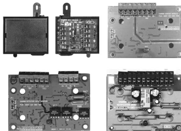
Typical MX Technology I/O Module Assemblies
