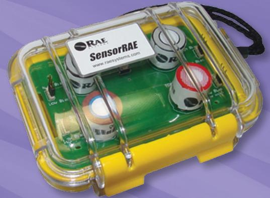
The SensorRAE is a compact waterproof conditioning station that keeps up to four RAE Systems' interchangeable electrochemical (EC) sensors warmed up and ready for immediate installation, calibration, and use in RAE Systems MultiRAE Plus and AreaRAE monitors. The SensorRAE offers users of these monitors the ability to broaden the spectrum of detectable compounds by having four additional EC sensors readily available in addition to the four EC sensors installed in the instrument.
