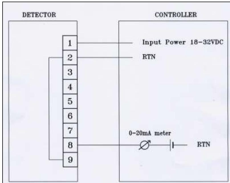
**Figure 11: 0-20mA Wiring Option 1 (Unisolated Sink 3-Wire)**
