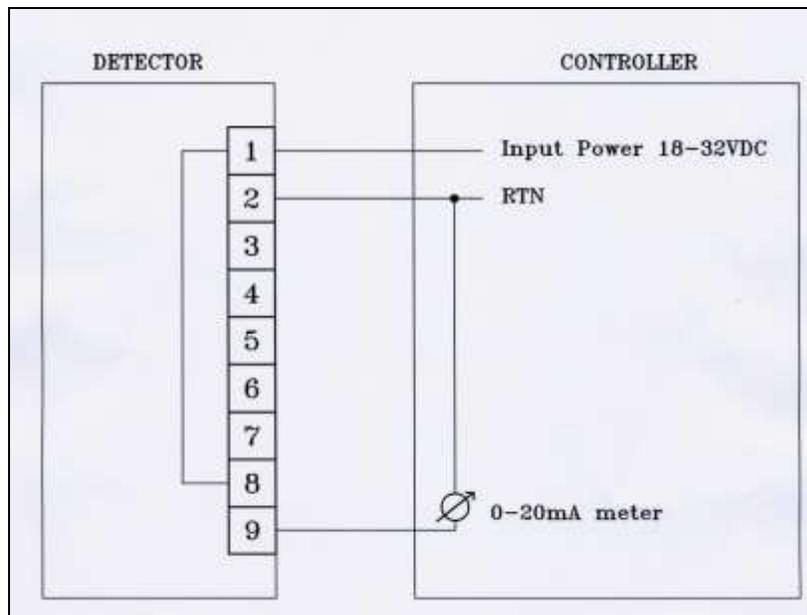
**Figure 10: 0-20mA Wiring Option 1 (Converted to Source 3-Wire)**
