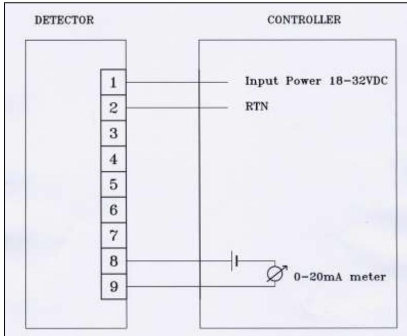
**Figure 9: 0-20mA Wiring Option 1 (Sink 4-Wire) - Default**
