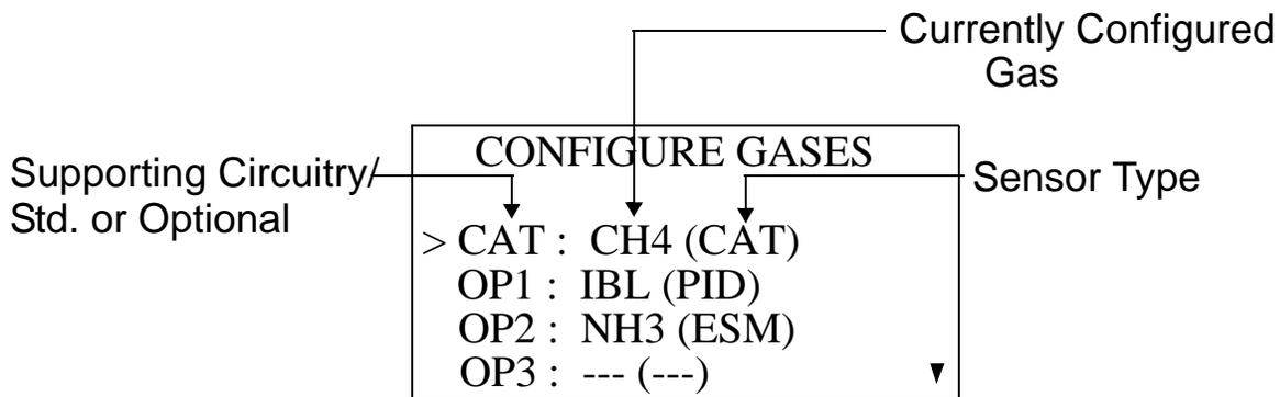
The four possible sensors are a catalytic sensor and three optional sensors. They are listed with the following information from left to right:
