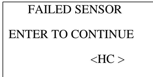
The buzzer and alarm LEDs activate in a double pulsing pattern. Press and release the POWER ENTER RESET button to reset the alarm and continue to the Calibration Mode Screen. Attempt to calibrate the infrared hydrocarbon channel again. If the failure continues, investigate the cause. See “Troubleshooting” on page 70
