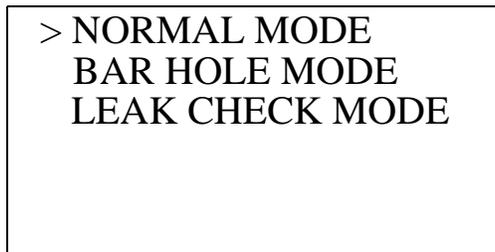
7. The cursor will flash in front of **NORMAL MODE**. Use the RANGE ▼ SHIFT button to move the cursor next to **LEAK CHECK MODE**.
