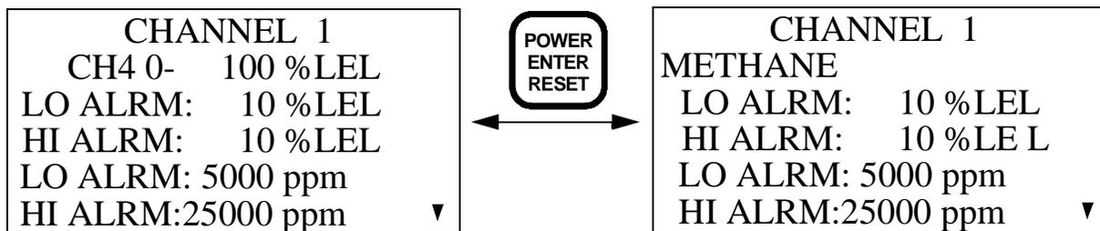
3. If the number of alarm settings is too many to display on one screen, a down arrow will appear in the lower right corner of the display indicating that there are additional alarm points. Press and release the RANGE ▼ SHIFT button to scroll down and display the remainder of the gas alarm settings for the displayed channel and again to return to the previous screen.
