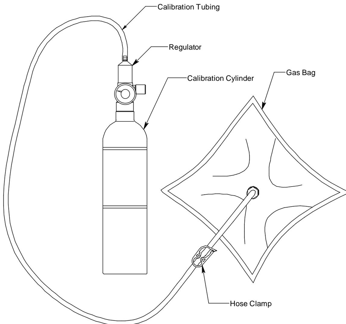
**Figure 23: Gas Bag Calibration Kit**
