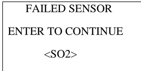
The buzzer and alarm LEDs activate in a double pulsing pattern. Press and release the POWER ENTER RESET button to reset the alarm and continue to the Calibration Mode Screen. Attempt to calibrate the ESM-01 channel again. If the failure continues, investigate the cause. See “Troubleshooting” on page 70
