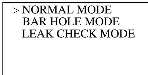
7. The cursor will flash in front of **NORMAL MODE**. Use the **RANGE ▼ SHIFT** button to move the cursor next to **BAR HOLE MODE**.
