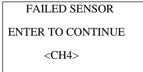
The buzzer and alarm LEDs activate in a double pulsing pattern. Press and release the POWER ENTER RESET button to reset the alarm and continue to the Calibration Mode Screen. Attempt to calibrate the TC channel again. If the failure continues, investigate the cause. See “Troubleshooting” on page 70
