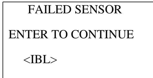
The buzzer and alarm LEDs activate in a double pulsing pattern. Press and release the POWER ENTER RESET button to reset the alarm and continue to the Calibration Mode Screen. Attempt to calibrate the PID channel again. If the failure continues, investigate the cause. See “Troubleshooting” on page 70
