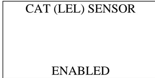
2. Use the AIR ▲ YES or RANGE ▼ SHIFT button to toggle to the desired setting.
