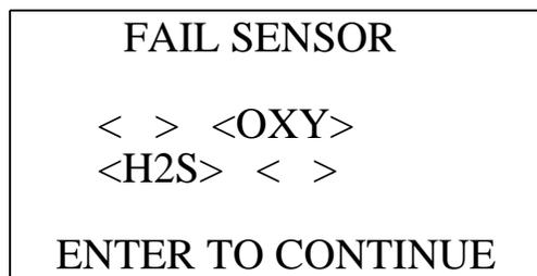
The buzzer and alarm LEDs activate in a double pulsing pattern. Press and release the POWER ENTER RESET button to reset the alarm and continue to the Calibration Value Screen for the PID channel. After calibrating the PID channel by following the instructions below, attempt to calibrate the standard channels again. If the failure continues, investigate the cause. See "Troubleshooting" on page 70
