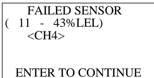
In the example above, the EAGLE 2 could have adjusted the reading as low as 11 %LEL and as high as 43 %LEL. Since the calibration gas value entered was 50 %LEL, the unit failed the span adjustment. The buzzer and alarm LED arrays activate in a double pulsing pattern. Press and release the POWER ENTER RESET button to reset the alarm and return to the Select Sensor Screen. Attempt to calibrate again. If the failure continues, investigate the cause. See “Troubleshooting” on page 70
