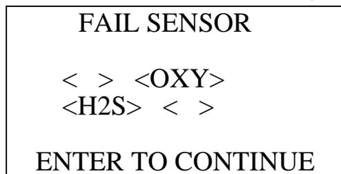
The buzzer and alarm LEDs activate in a double pulsing pattern. Press and release the POWER ENTER RESET button to reset the alarm and continue to the Calibration Value Screen for the TC channel. After calibrating the TC channel by following the instructions below, attempt to calibrate the standard channels again. If the failure continues, investigate the cause. See “Troubleshooting” on page 70
