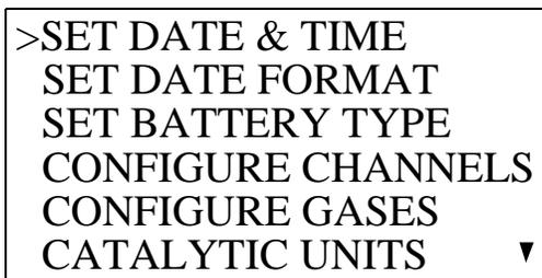
6. Use the RANGE ▼ SHIFT button to move the cursor down the menu to CONFIGURE GASES.
