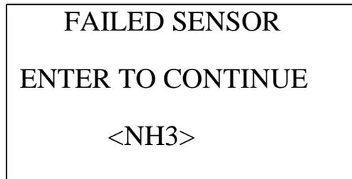
The buzzer and alarm LEDs activate in a double pulsing pattern. Press and release the POWER ENTER RESET button to reset the alarm and continue to the Calibration Mode Screen. Attempt to calibrate the ESM-01 channel again. If the failure continues, investigate the cause. See “Troubleshooting” on page 70.
