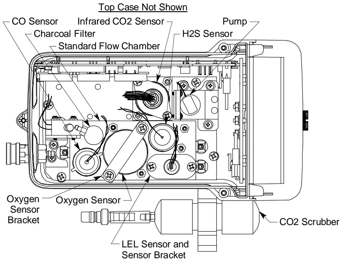
**Figure 38: Typical Infrared CO<sub>2</sub> Sensor Location**
