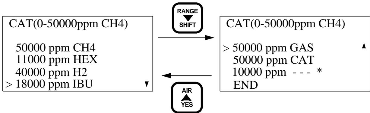
All of the gases except for the one with the asterisk (\*) next to it are pre-defined. The gas with the asterisk next to it is user defined. The user defined gas can be used if the desired gas is not one of the pre-defined gases. Below is a brief description of each choice.
