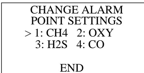
8. Move the cursor next to the oxygen channel. Press and release POWER ENTER RESET.
