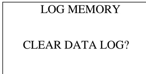
2. If you do not want to clear the data logger memory at this point or at Step 3 below, press and release the DISPLAY ADJUST NO button. The unit will return to Measuring Mode.
