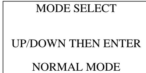
Use the AIR ▲ YES or RANGE ▼ SHIFT button to display the mode you wish to enter and press and release the POWER ENTER RESET button.
