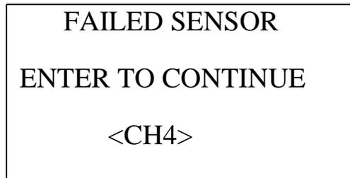
The buzzer and alarm LEDs activate in a double pulsing pattern. Press and release the POWER ENTER RESET button to reset the alarm and continue to the Calibration Mode Screen. Attempt to calibrate the infrared methane channel again. If the failure continues, investigate the cause. See “Troubleshooting” on page 70
