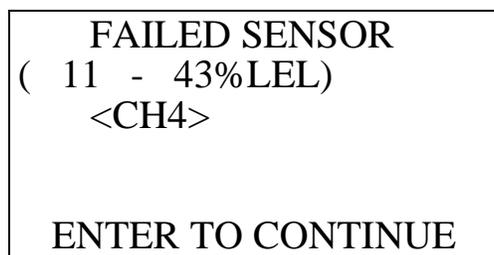
In the example above, the EAGLE 2 could have adjusted the reading as low as 11 %LEL and as high as 43 %LEL. Since the calibration gas value entered was 50 %LEL, the unit failed the span adjustment. The buzzer and alarm LED arrays activate in a double pulsing pattern. Press and release the POWER ENTER RESET button to reset the alarm and return to the Select Sensor Screen. Attempt to calibrate again. If the failure continues, investigate the cause. See “Troubleshooting” on page 70
