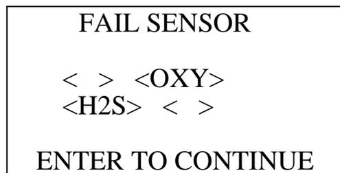
The buzzer and alarm LED arrays activate in a double pulsing pattern. Press and release the POWER ENTER RESET button to reset the alarm and return to the Calibration Mode Screen. Attempt to calibrate again. If the failure continues, investigate the cause. See "Troubleshooting" on page 70
