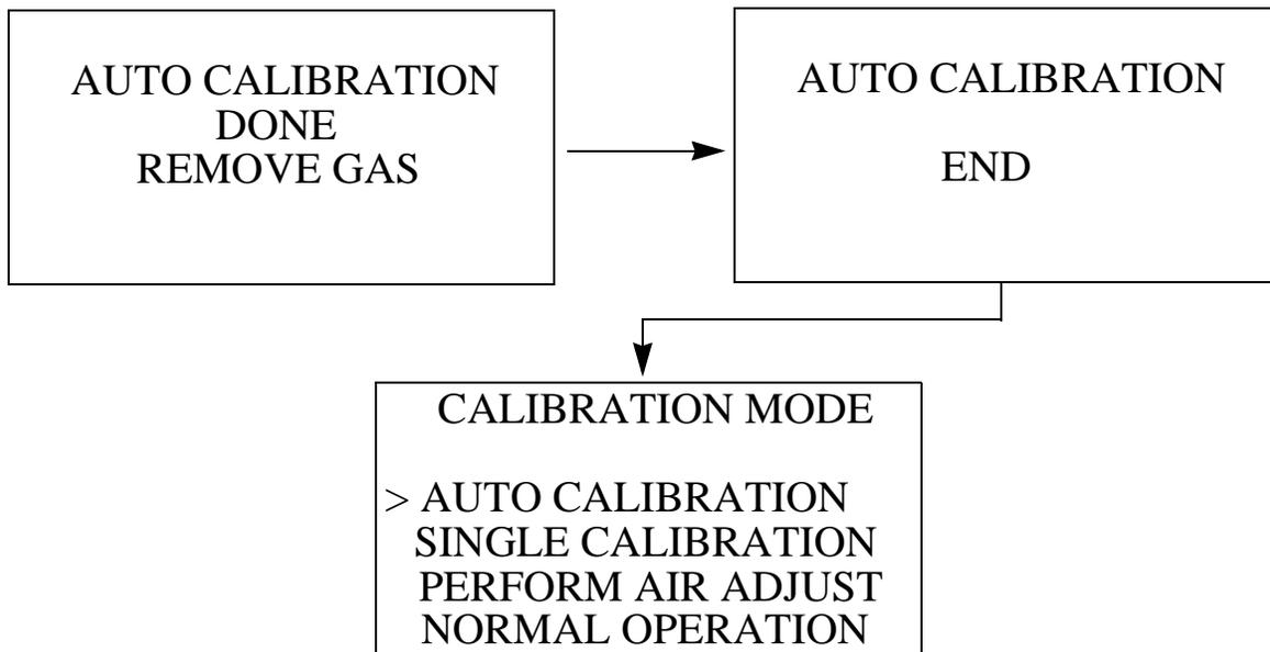
If the infrared CO<sub>2</sub> channel cannot be adjusted to the proper value, a screen displays that indicates a calibration failure and indicates that the infrared CO<sub>2</sub> sensor failed to calibrate.
