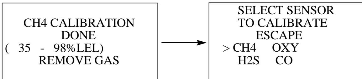
In the example above, the EAGLE 2 could have adjusted the reading as low as 35 %LEL and as high as 98 %LEL.
