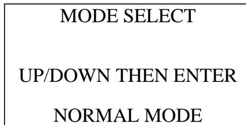
Use the AIR ▲ YES or RANGE ▼ SHIFT button to display the mode you wish to enter. If you have not made a selection after 20 seconds, the instrument will begin to beep and the LEDs will begin to flash. They will continue until you make a selection.
