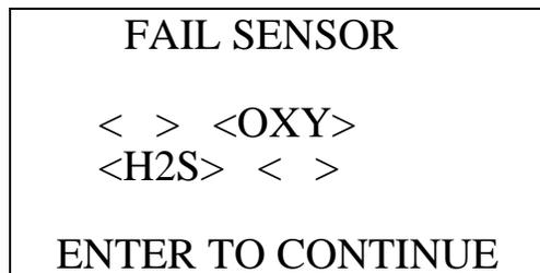
The buzzer and alarm LEDs activate in a double pulsing pattern. Press and release the POWER ENTER RESET button to reset the alarm and continue to the Calibration Value Screen for the infrared methane channel. After calibrating the infrared methane channel by following the instructions below, attempt to calibrate the standard channels again. If the failure continues, investigate the cause. See “Troubleshooting” on page 70.
