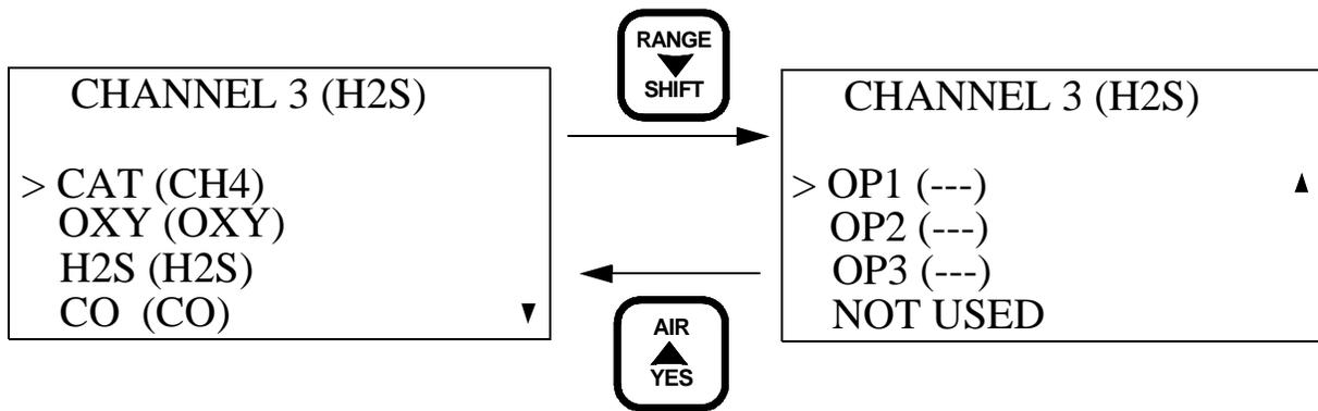
5. Use AIR ▲ YES and RANGE ▼ SHIFT to move the cursor next to the desired configuration for the selected channel. In the example below, the cursor has been moved next to the **NOT USED** selection.
