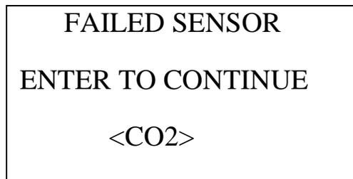
The buzzer and alarm LEDs activate in a double pulsing pattern. Press and release the POWER ENTER RESET button to reset the alarm and continue to the Calibration Mode Screen. Attempt to calibrate the infrared CO<sub>2</sub> channel again. If the failure continues, investigate the cause. See “Troubleshooting” on page 70
