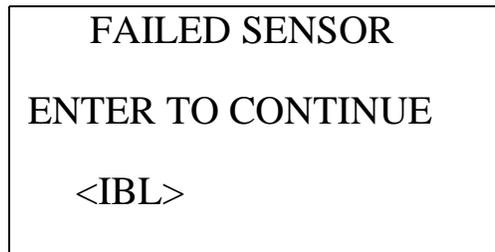
The buzzer and alarm LEDs activate in a double pulsing pattern. Press and release the POWER ENTER RESET button to reset the alarm and continue to the Calibration Mode Screen. Attempt to calibrate the PID channel again. If the failure continues, investigate the cause. See “Troubleshooting” on page 70
