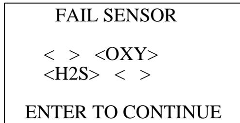
The buzzer and alarm LEDs activate in a double pulsing pattern. Press and release the POWER ENTER RESET button to reset the alarm and continue to the Calibration Value Screen for the ESM-01 channel. After calibrating the ESM-01 channel by following the instructions below, attempt to calibrate the standard channels again. If the failure continues, investigate the cause. See “Troubleshooting” on page 70
