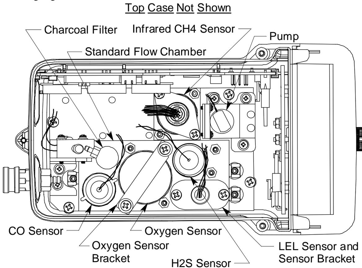
**Figure 40: Typical Infrared Methane Sensor Location**
