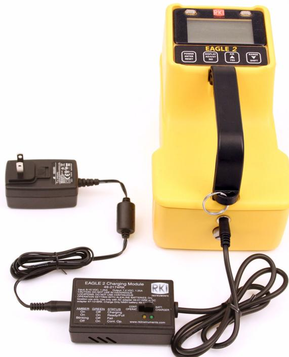
Figure 18: Connecting the EAGLE 2 to the Charger
