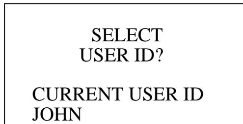
The user ID provides a way to identify the EAGLE 2 user during a data logging session. If the user ID is changed during an operating session, a new data session is initiated with the new user ID attached to it. This allows you to change the user ID during operation and have each user ID that was used during an operating session saved for the corresponding data. See the Eagle 2 Data Logger Management Program Operator’s Manual for a detailed description of data logging and the user ID.
