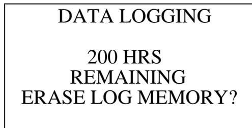
To return to Measuring Mode while at the Data Logging Screen, press and release the DISPLAY ADJUST NO button.
