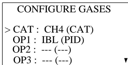
8. Use RANGE ▼ SHIFT to move the cursor down the menu to the PID sensor.
