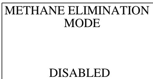
The standard setup for methane (CH<sub>4</sub>) does not support methane elimination. When applicable, use this screen to enable and disable the methane elimination feature. See “Appendix J: Methane Elimination Mode” for more discussion of the methane elimination feature.
