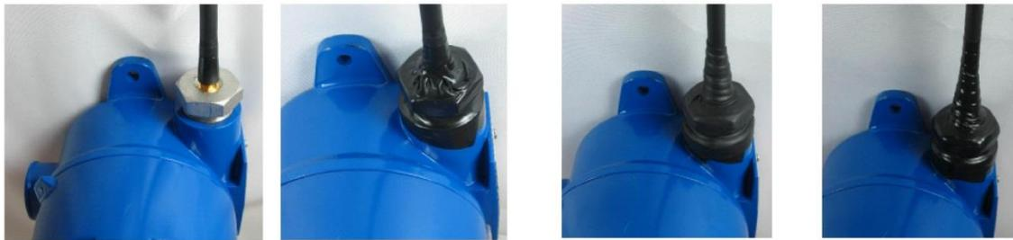
Figure 65 Water-proofing Antenna Connections
