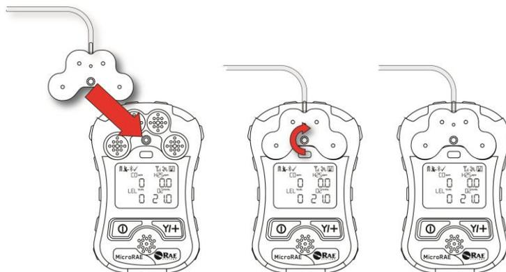
1. Align the Calibration Adapter's main body with the indented area around the MicroRAE's gas inlets.
