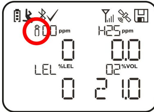
A bump test is required if the defined period of time between bump tests has been exceeded. This interval is set by an administrator using ProRAE Studio II.
