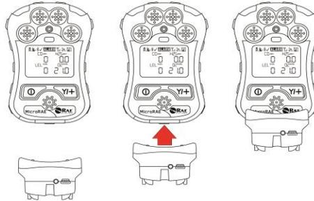
**Align the Travel Charger with the middle of the MicroRAE and press it until it is firmly attached.**
