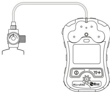
4. Connect the calibration adapter to the calibration gas.
