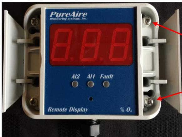
2) Loosen the 4 screws to separate the front panel from the case.
