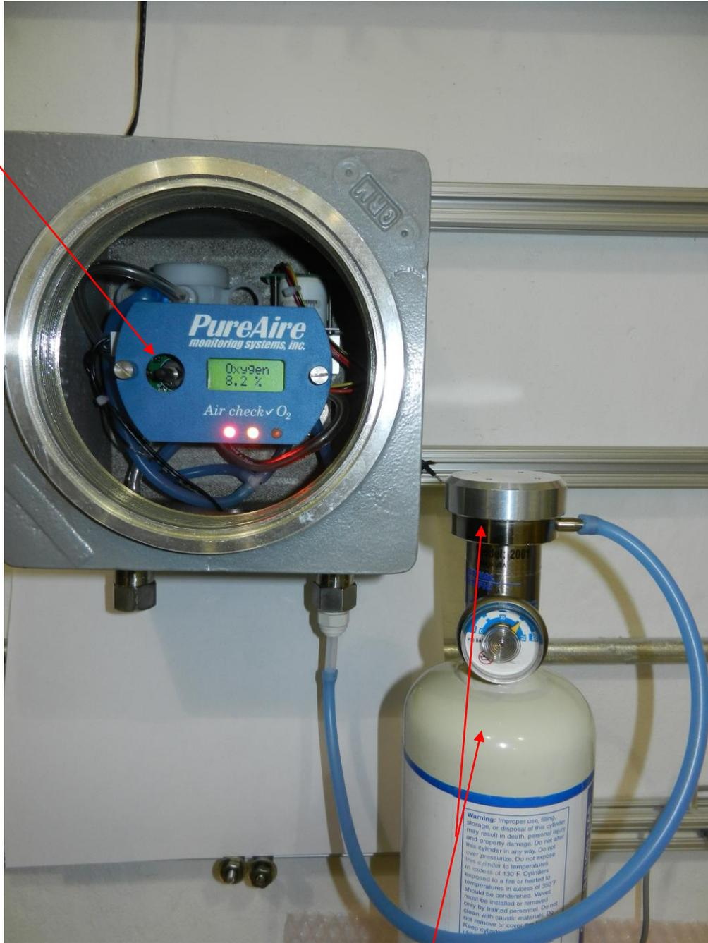
Oxygen span gas
