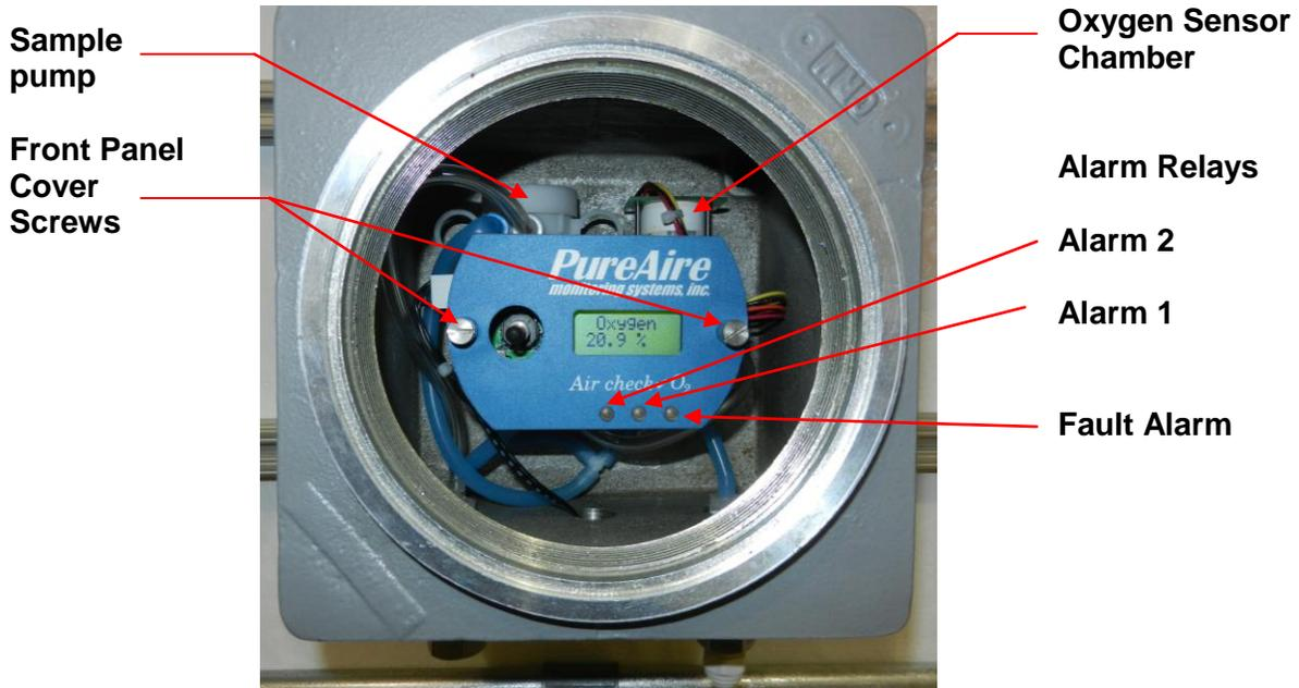
O<sub>2</sub> monitor with front cover removed
