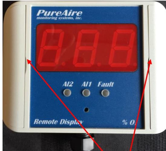
1) Open the two side doors to expose the front panel screws.
