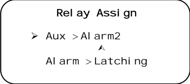
Relay mode will be always "Latching". Once decided press EXIT button to return to main screen. When AUX relay assigned to ALARM3, Digital Input port will be monitored on the panel and AUX relay will be activated once the digital input activated by external device.
