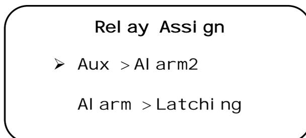
Press MENU button to change AUX relay assignment. A cursor will be activated on the screen and you can change assignment via using UP and DOWN buttons. Once complete press EXIT button to save and return the screen.
