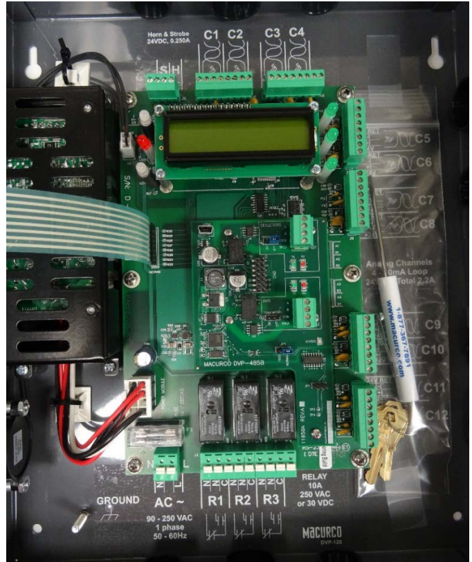
Figure 3-4 DVP-120 Internal View and DVP-120B with DVP-485 Modbus Adapter
