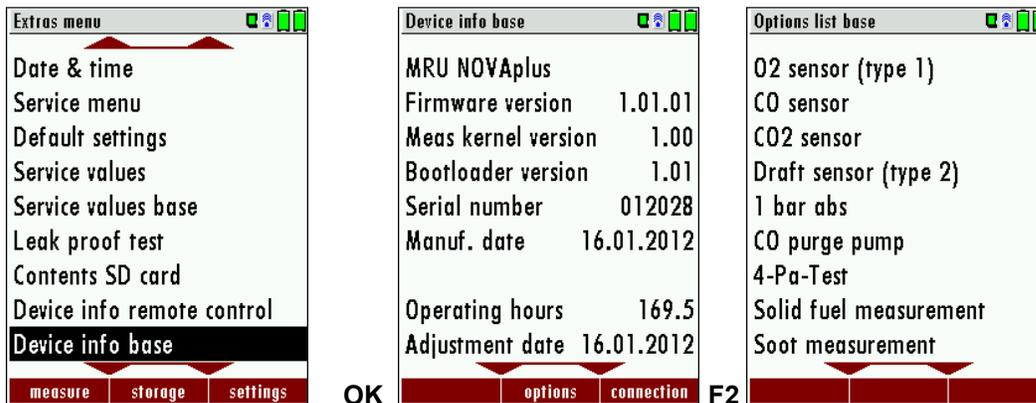
Use the F2 button to see the installed options of the base unit.
