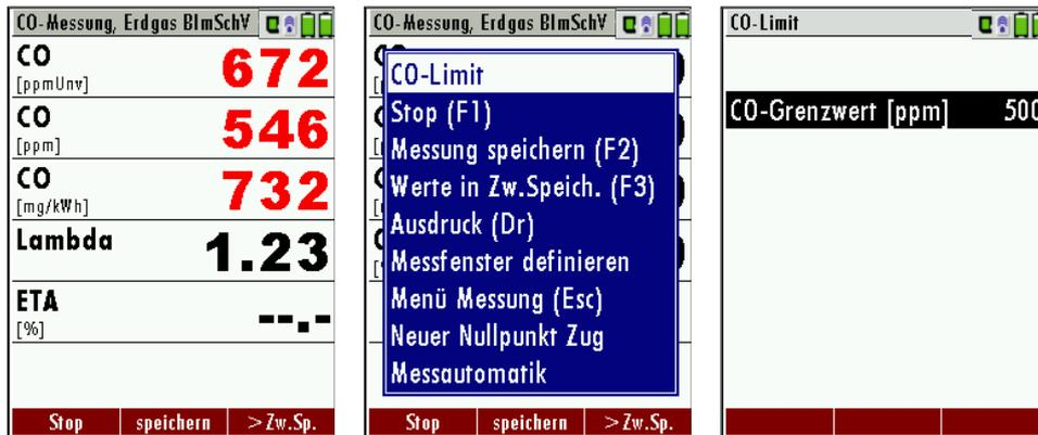
If the CO limit value is exceeded, the color of the measured CO values changes (red).
