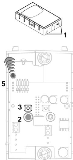
1. Back out set screws along bottom edge of enclosure cover and remove cover
