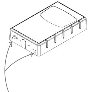
Once lid is closed, insert set-screws to lock enclosure.
