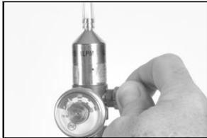
To start the flow of gas, turn the regulator knob in a counterclockwise direction.
