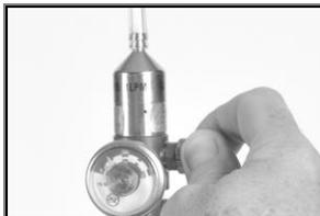
To stop the flow of gas, turn the regulator knob in a clockwise direction and tighten.
