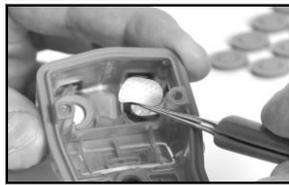
Guide the new filter— adhesive side down—into the filter opening.
