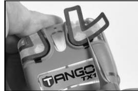
Guide the new barrier—adhesive side down—onto the case top.
