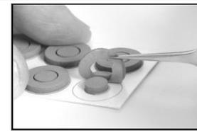
Grip the gasket ring lightly with the tweezers; peel the gasket ring from the packet.
