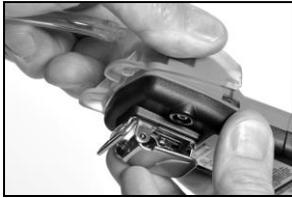
Place the calibration cup over the case top; align its top groove with the small ridge at the top of the instrument. Press down to secure the cup in place; a click will sound. Visually inspect the calibration cup to ensure its edges along the top and sides align with the case top edges.
