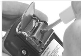
Guide the screwdriver through the clip's hole and into the screw head. Turn clockwise to tighten.
