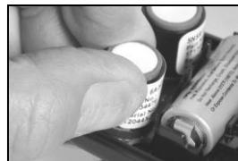
Secure the sensor in place by applying gentle pressure to the sides of the sensor case. Do not touch the sensor's white membrane.
