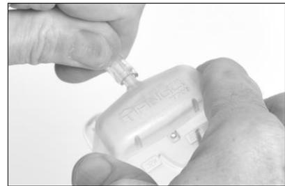
Connect the other end of the tubing to the calibration cup. Proceed with the instruction set below for the desired task: calibration or bump testing.
