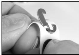
The plates are adhered to a paper backing. Bend the paper backing to separate the plate.
