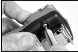
Using a torx screwdriver, remove all four screws from the case bottom; set aside the screws.
