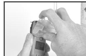
To remove the calibration cup, lift up from the cup's tabs. Set aside or store for future use.
