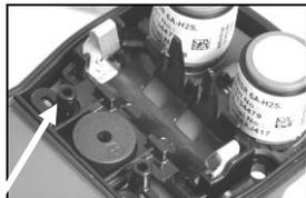
The instrument's interior power button is located below the battery cradle and to the left of the speaker (see arrow above).
