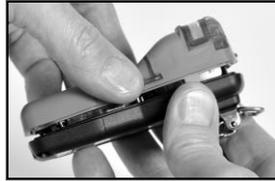
Hold the case bottom near the upper screw holes; lift the case top slightly to separate the top and bottom.
