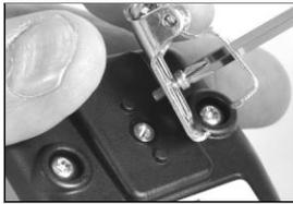
To attach the clip cover, place the screw through the center hole of the clip back.
