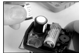
Lift the sensor to remove it.
