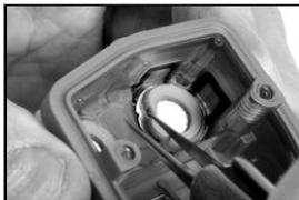
Inside the case top, grip the gasket and underlying sensor filter with the needle-nose tweezers; peel to remove.
