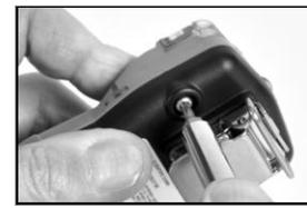
Using a torx screwdriver, insert and tighten each of the four screws into the case bottom.
