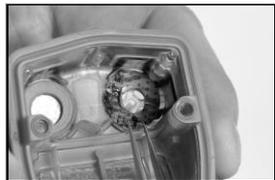
Remove any remnants of the adhesive, filter, or gasket.
