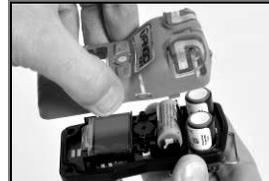
Continue to lift the case top straight up to remove it and to avoid unintentionally loosening the sensors.
