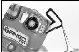
Using a finger or needle-nose tweezers, peel off the dust barrier and discard.
