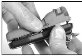
Lower the case top assembly onto the case bottom. Use a straight-down motion to guide the sensors into the sensor barrels.
