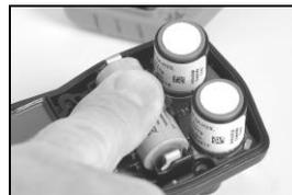
Orient the replacement battery so the positive and negative ends align with the "+" and "-" cradle markings, respectively. Place the new battery into the cradle negative end first.
