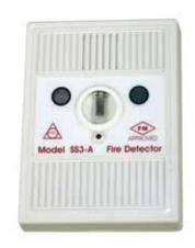
The Model SS3-A (latching fire alarm relay) and SS3-AN (non-latching Fire Alarm relay) retain outstanding fire and flame detection capabilities in a non explosion-proof, ABS housing. This detector senses radiant energy in the ultraviolet (UV), visible and wide band infrared™ (IR) spectrum. The radiant energy from all types of flaming fires will alert the detector to their presence.
