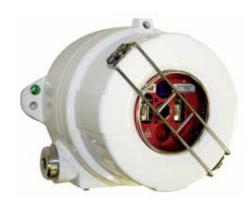
The SS4 is a hazardous area certified flame detector for the detection of hydrocarbon (SS4-A2) and non-hydrocarbon fires (SS4-AS2). This multispectrum detector senses radiant energy in the ultraviolet (UV), visible and wideband infrared (IR) spectrum. The radiant energy from all types of flaming fires will alert the detector to their presence. The field of view is the widest in the industry with 120° field of view with a range of 60 feet. This means more hazard can be covered by each detector.
