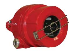
A high-speed microprocessor based fire detection and process control system specially designed for liquid and powder coating applications, the Fire Sentry FS System 10 quickly detects the presence of a flame, reacts by initiating a shutdown of the electrostatic finishing process in a matter of milliseconds; and effectively interrupts the fire before residues and wet paint films can ignite.
