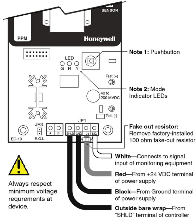
**Electrical Power:** 24 VDC regulated, 30 mA. With an ATMOS® equipped enclosure the current draw is 400 mA max.
