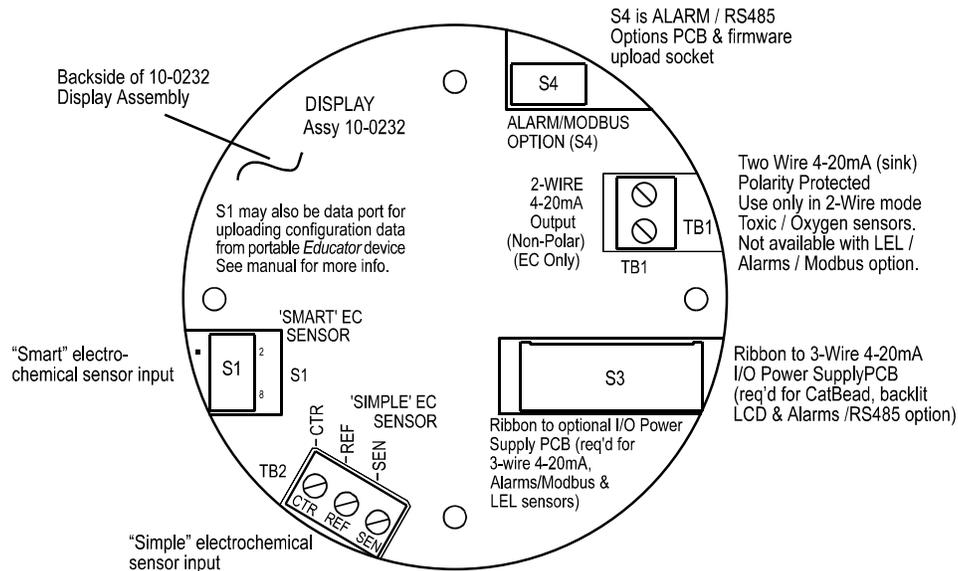
**FIGURE 1: TRANSMAX / EC DISPLAY BOARD**
