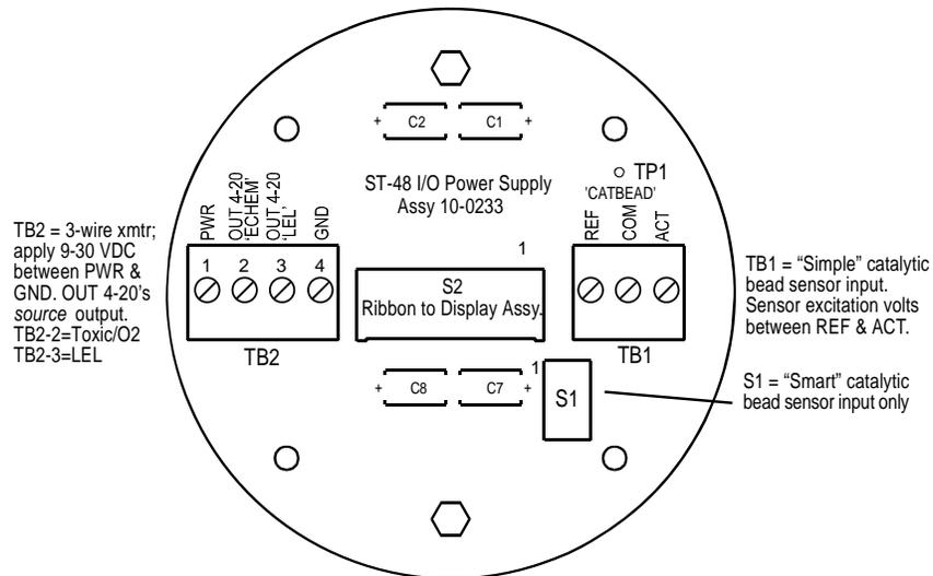
FIGURE 2: TRANSMAX II I/O Power Supply Board
