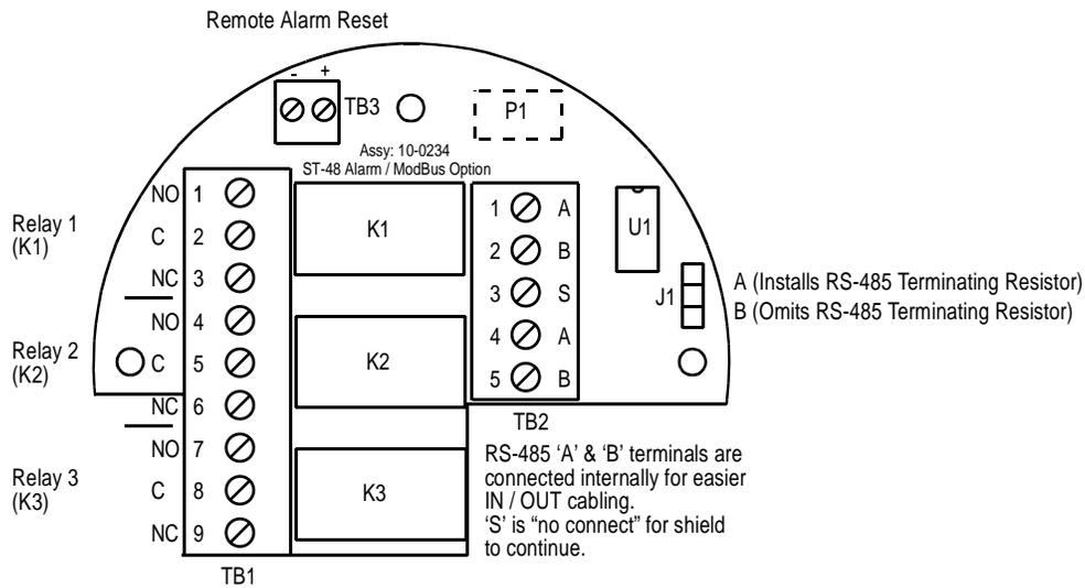
**FIGURE 3: TRANSMAX II Alarm / MODBUS Board**
