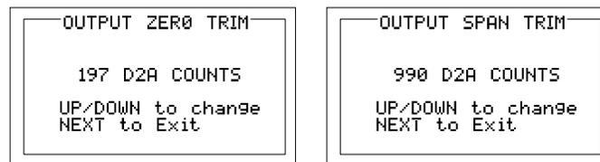
Figure 12: Output ZERO / SPAN Trim Menus
