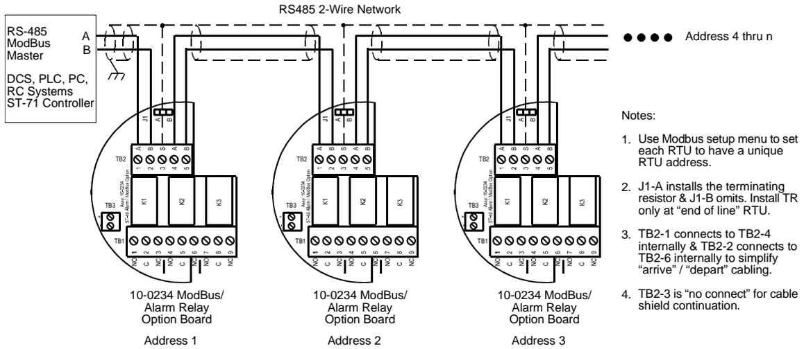
FIGURE 4: TRANSMAX II Alarm / MODBUS Board
