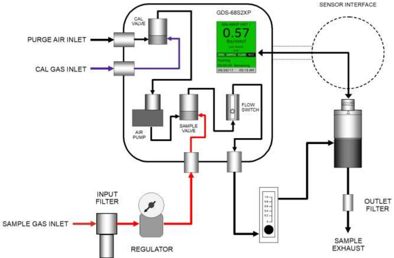
Figure 6-1: Functional Block Diagram
