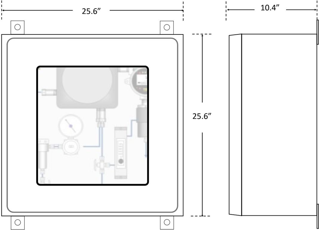
Figure 19-1: GDS-68S2XP Dimensions With Wall-Mount Kit
