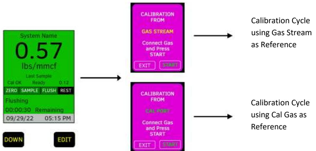
Figure 11-1 Manual System Calibration
