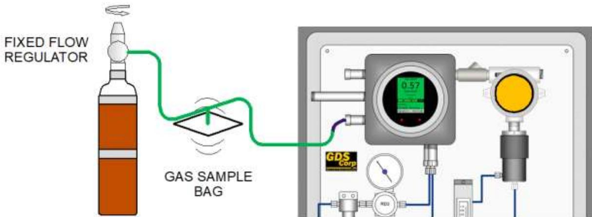
Figure 10-2: Calibration Setup (Fixed Flow Regulator)
