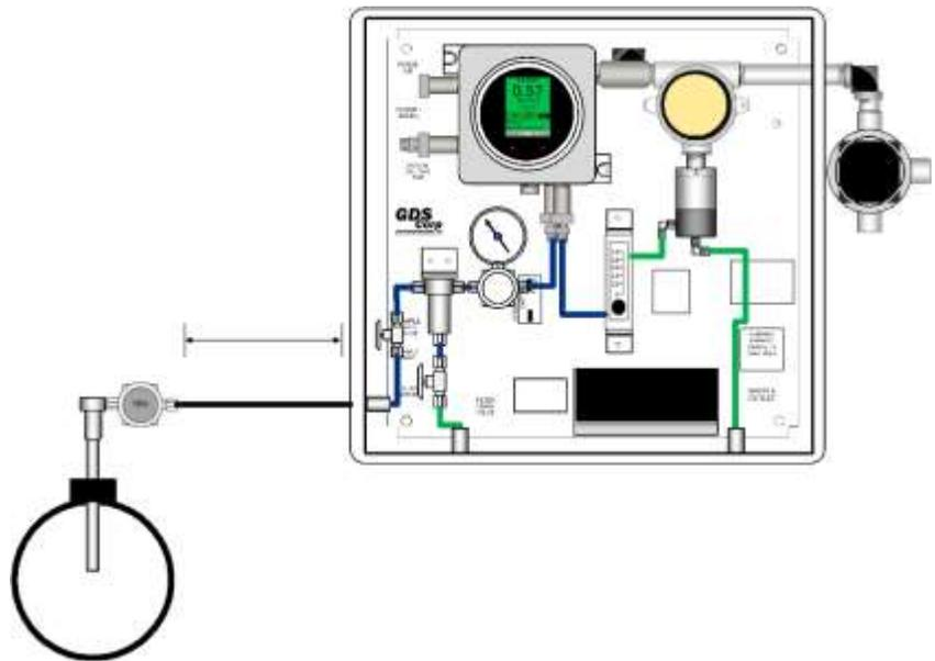
GDS Corp recommends installing a low-volume high-pressure regulator / filter at the point where the gas is extracted from the pipeline. This will minimize the pressure in the line between the gas extraction point and GDS-68S2XP and further reduce the total volume of gas stored in the sample line.
