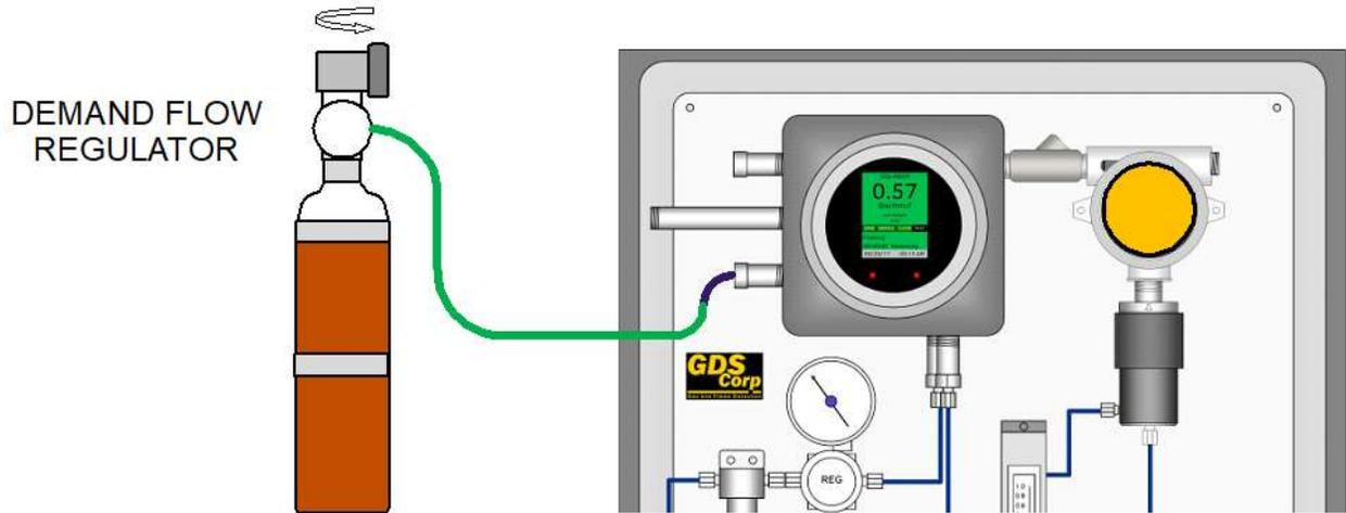
Figure 10-1 Calibration Setup (Demand Flow Regulator)
