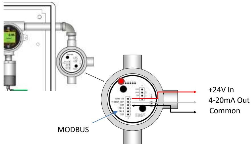
Figure 7-1 GDS-68S2XP Wiring Junction Box
