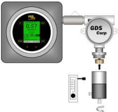
Step 6: Install the new sensor by aligning the arrow on the sensor label with the engraved arrow on the sensor head and pushing straight up.
