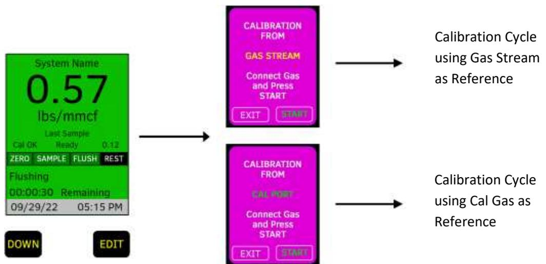
Figure 11-1 Manual System Calibration
