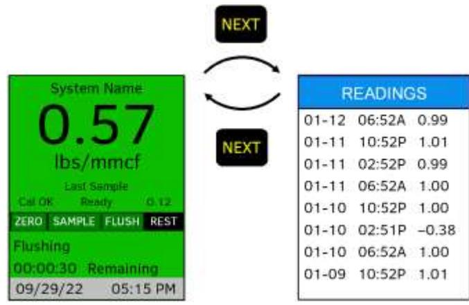
Figure 9-3 Last Readings Screen
