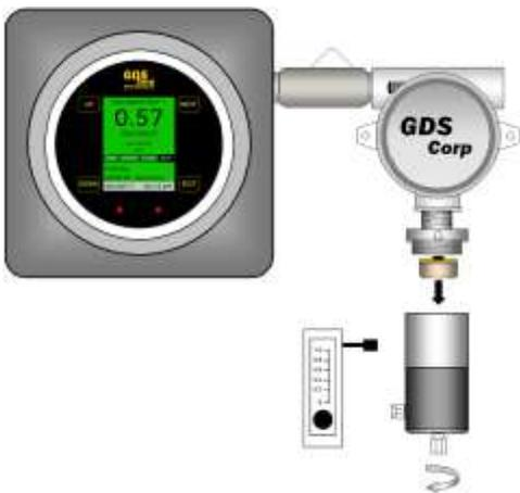
Step 3: Unscrew the flow cell + sensor head cover being careful not to dislodge the sensor element.
