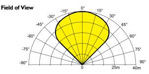
To meet the requirements of EN54:10 dause 5.4, where the ratio of the response points Dmax: Dmin should not exceed 1.41, the horizontal and vertical viewing angles max should not exceed  $\pm 30^{\circ}$ .
