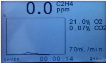
The x-axis of the graph represents time elapsed. The y-axis of the graph displays the range of the concentration in % for CO<sub>2</sub> and O<sub>2</sub>, and the dynamic range is labeled at the top. The y-axis scale is set by the highest value shown in the active display.
