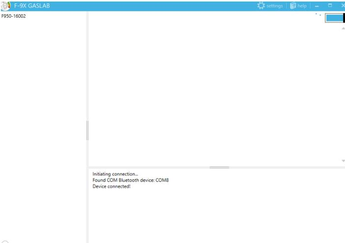
4. Once connected, your device serial number should appear in the upper left hand corner of the window, click on the serial number, you are now ready to interact with the F-960 Ripen It! Click on the grey and blue square in the upper right hand corner to dis-connect or re-connect.
