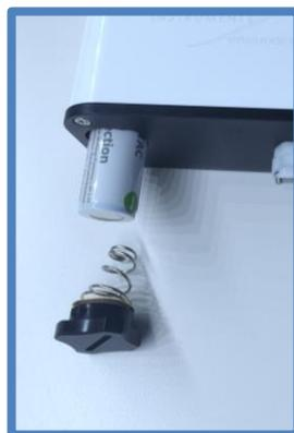
To remove the batteries, twist the battery compartment cap, located on the bottom of the case. The cap can be twisted with fingers or a screw-driver to tighten or loosen it. Take care when removing batteries, as the cap is
