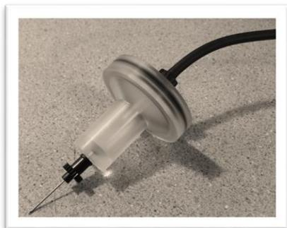
After measuring, the water in the PolarCept filter will become saturated with trapped interfering gases and should be replaced with fresh distilled water. Saturation rates will depend on the amount of interfering gases present in the sample environment. The table below shows example saturation times when measuring headspace of bananas (with a maturity index of 5) in Continuous Mode. This sample contains various mixed hydrocarbons, ethylene and VOCs.
