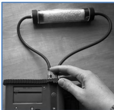
Next, verify the set zero calibration by measuring ambient air. Run the set zero calibration again if the verification is not successful.
