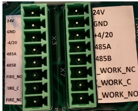
**Figure 5-2: Arrangement and Functions of Mounting Connection Terminals**
