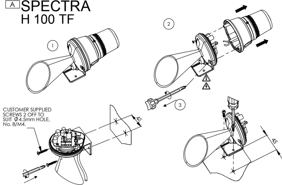
CUSTOMER SUPPLIED SCREWS 2 OFF TO SUIT Ø 4.5mm HOLE, No. 8/M4.
