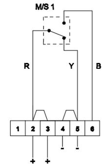
**Unit in 'Operated condition' (button pushed in)**
