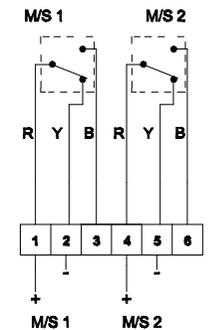
**Unit in 'Operated condition' (button pushed in)**
