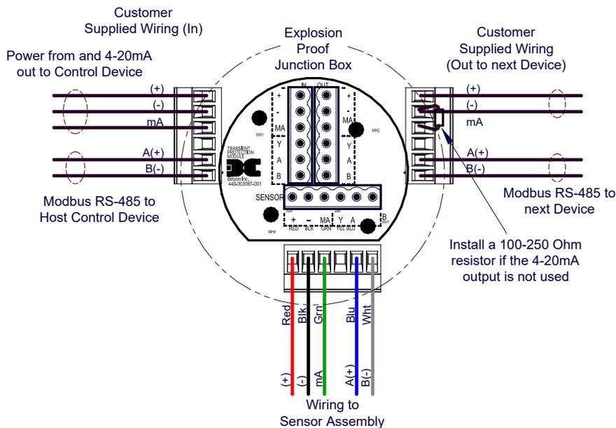
**Figure 13** Sensor Wire Connections
