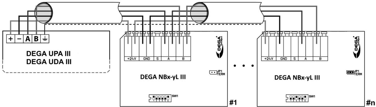
**1. Installation of wiring for RS485**
