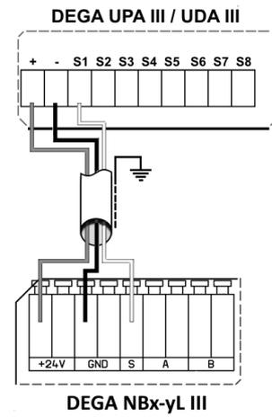
**4. Connecting the sensor via RS485 to the controller DEGA UPA III/UDA III**
