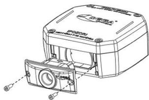
This activity must not be performed when the sensor is energized.
