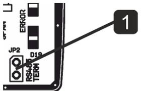
According to the RS485 specifications, the last device on the bus must be ending with a terminating resistor 120R. Plug a jumper on the JP2 connector of the last device on the bus to include the 120R terminating resistor. In the default configuration the jumper connector is not plugged.
