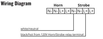
Figure 1 Strobe and Horn operate together (position jumpers as shown below)
