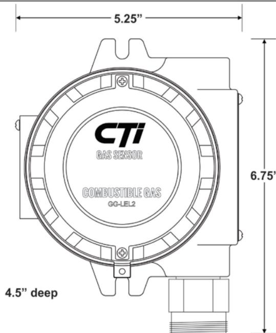
**Figure 1: Mounting Dimensions**
