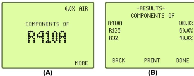
Figure 4-8. Sample Test Results for Pure Blend Refrigerant with Incorrect Component Ratios
