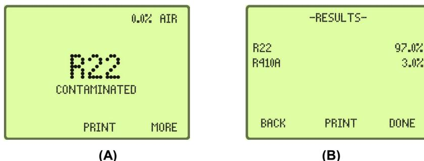
Figure 4-4. Screens Showing Sample Test Results
