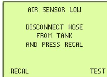
**Figure 5-5. Sample Screen Showing Air Sensor Low Message**
