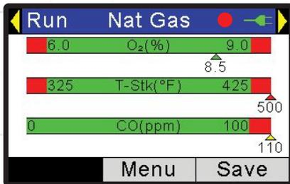
Using color-coded arrows, Tune-Rite™ shows which readings are in range (green), unstable (yellow) or out of range (red).
