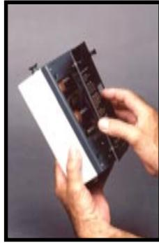
The cell is keyed to ensure proper alignment into the instrument. When installed, the circuit board of the cell should be flat with the bottom of the instrument. Push up on the clear window at the back of the instrument to eject the cell.
