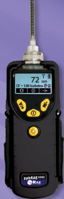
The compact ppbRAE 3000 is a comprehensive VOC gas monitor and datalogger for hazardous environments. The ppbRAE 3000 is the most advanced handheld VOC monitor available for parts-per-billion detection. This third-generation patented PID device monitors VOCs using a photoionization detector with a 9.8 eV, 10.6 eV UV-discharge lamp.
