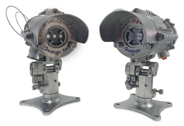
The SafEye Quasar 960 is part of he innovative SafEye Quasar open path gas detector series. The detector provides ultraviolet technology continuous monitoring for toxic ammonia ( $NH_3$ ) gas at very low concentrations, up to 95 percent obscuration, featuring advanced wide area coverage with long range detection up to 200 ft. (60 m) and high speed response in under 10 seconds.
