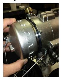
Now that the detector and flash source have been attached to the mounting brackets it is time to wire them up. But first you must remove the back cover from the unit. Simply screw the unit off counter-clockwise revealing the wiring terminals.
