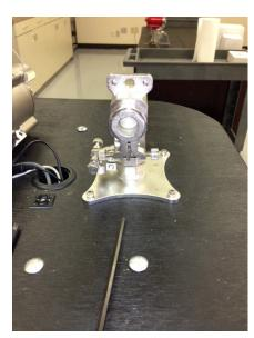
The next step in the process is to attach the mounting brackets (pn: 888270) to whatever surface according to the specifications of the project. Please note the orientation of the detector mount so that the mounting brackets are pointed in the correct direction.
