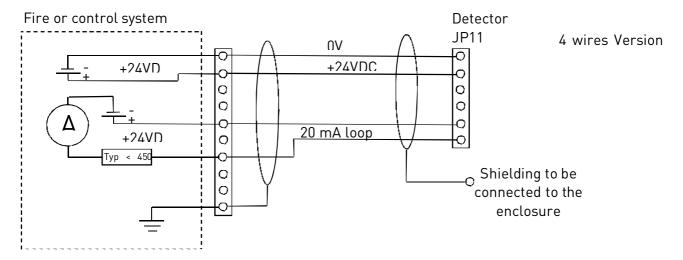
When using a 4 wires connection, the current loop is provided by the input module or PLC. The loop (L + and L-) is optically isolated from the detector. 4-20mA or 0-22mA input module of the PLC has to power up the current loop with, at least 8V at the terminal level, for 22 mA. This reduces the resistance of the loop as defined in the relationship below.
