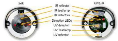
Alarms information is indicated by the flashing of a red LED in the communication head and of two LEDs located in front of the detection cartridge. Information and detector status is also available via the remote control TLU 600/610 display.
