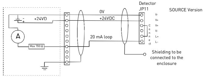
For a standard 3-wires connection, the 20mA current loop must be supplied with 24 V at terminal L+. To proceed, connect the 3 (V +) and 5 (L +) terminals at the terminal block level of the device.
