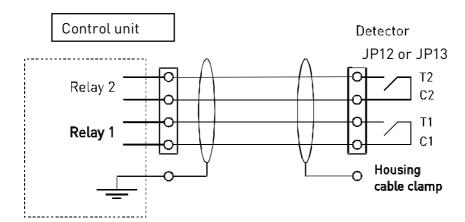
The two relays can be configured normally closed or normally open. If normally open, the relays are opened when they are not powered (power loss).
