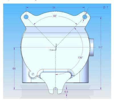
Figure 3: Drilling dimensions for support fixing.
