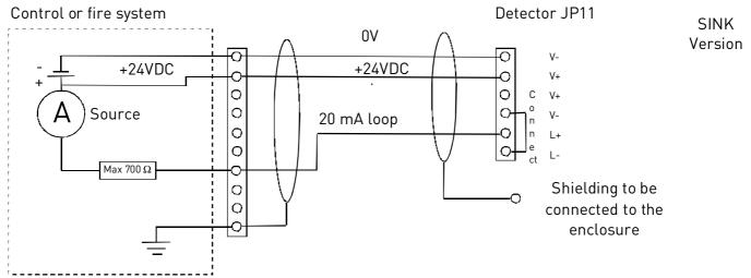
For a standard 3-wires connection in sink mode, the 20mA current loop must be supplied with a PLC. The current return must be connected to the 0V at the level of the L- terminal. To proceed, please connect the 4 (V-) and 6 (L-) terminals at the terminal block level of the devise.
