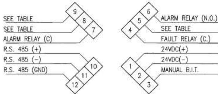
**Figure 7: Wiring Terminals**
