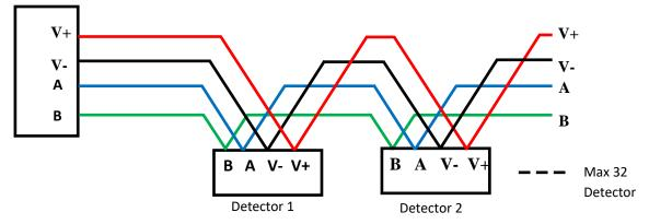
**Diagram 1: Panel to detector connections**
