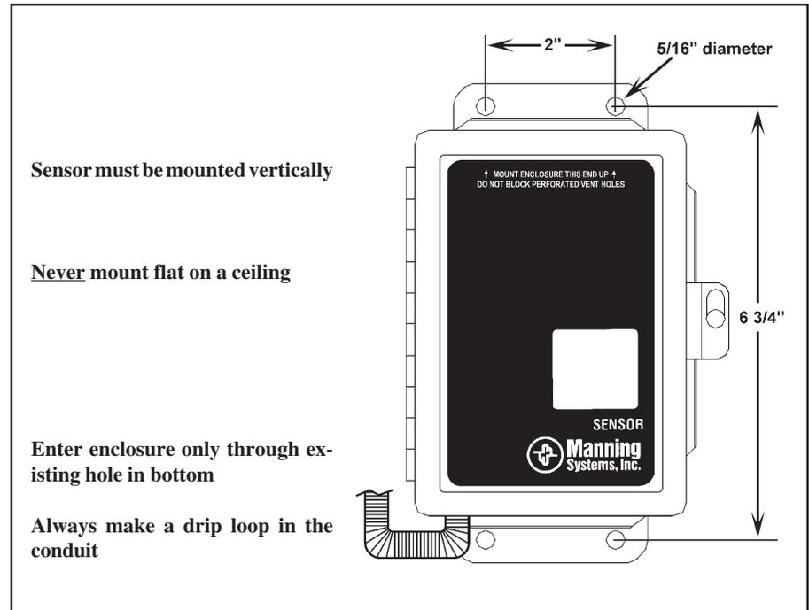
Figure 1: Mounting dimensions for the EC-F2 Sensor
