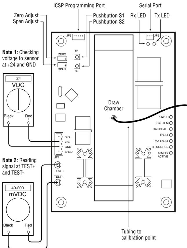
**Note 1:** Checking voltage to sensor at +24 and GND
