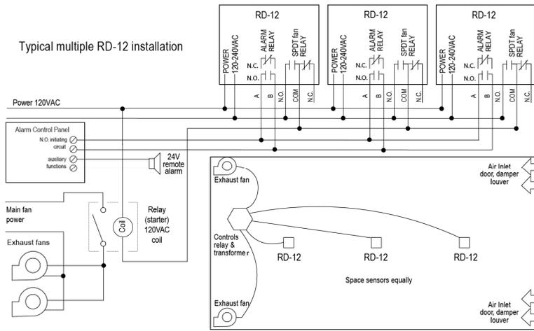
Alternate connection to alarm control panel
