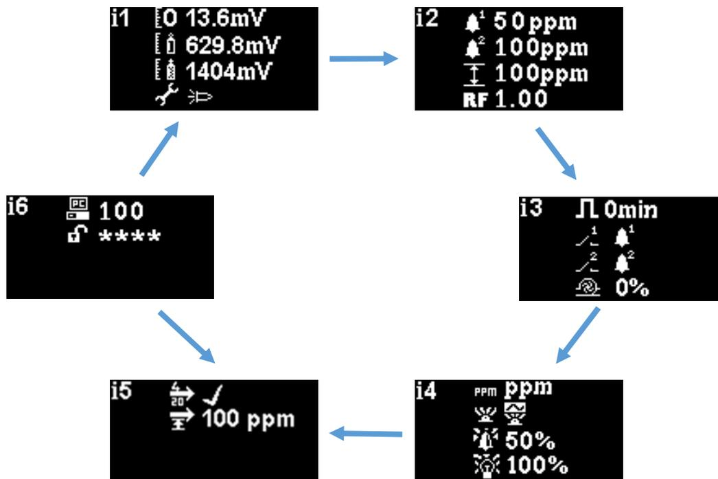
To access the settings menus, press the **Right** key from the Normal Running Mode screen. If a passcode has been set, the Lock screen will be displayed. Otherwise, the **i1** menu will be displayed.
