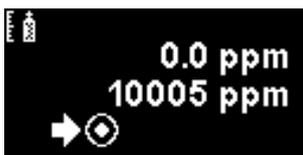
The top value is the live ppm reading from the Falco (based on previous calibration)
