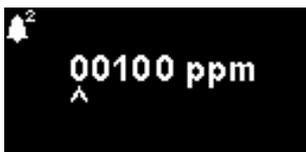
Used to set the ppm level at which Alarm 2 (red) is triggered. When accessed, the screen displays the current level.
