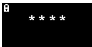
The Lock screen is displayed if a password number has been specified (see menu **i6**). It protects the instrument from unauthorised adjustment - the menus (see below), cannot be accessed until the correct number has been entered.
