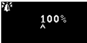
Used to set the brightness of the Status Light during alarm conditions, from 0 to 100%, or to AUTO mode.
