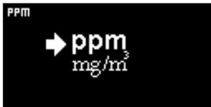
Used to change the detection units from the default of ppm to milligrams per meter cubed ( $\text{mg}/\text{m}^3$ ).
