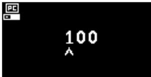
Used to select a Modbus slave address.
