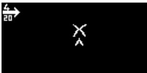
Used to turn the 4mA to 20mA output on and off.
