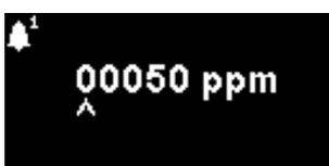
Used to set the ppm level at which Alarm 1 (amber) is triggered. When accessed, the screen displays the current level.
