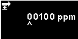
The lower limit of the 4mA to 20mA output range, mapped to 4mA, is 0ppm. This option is used to set the upper limit, mapped to 20mA.
