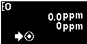
The top value is the live ppm reading from the Falco (based on previous calibration)
