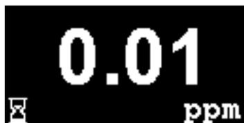
The screen then appears continuously and shows the PID reading and units. The Status Light colour depends on the status.
