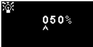
Used to set the brightness of the Status Light during normal operation, from 0 to 100%, or to AUTO mode.
