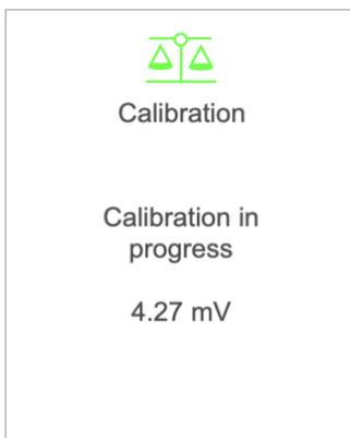
Once the instrument has stabilised, the calibration will finish. To confirm calibration, press ok, again, you can abort at this stage if required. The calibration will then save to the instrument. This calibration will automatically be added to the user load list.
