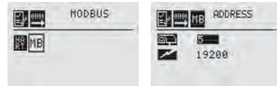
Figure 184. Modbus Configuration Display Screen
