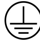
Figure 4. Equipment Earth (Ground) Point
