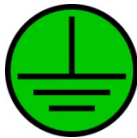
Figure 3. Protective Earth (Ground) Point
