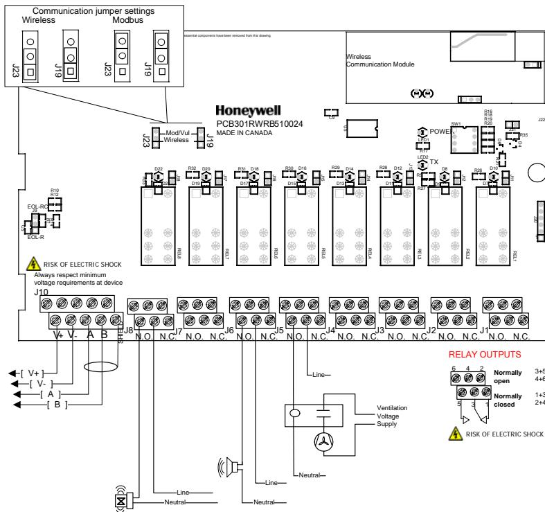
Wiring of communication lines depends on the communication jumper positions: If the jumper is in Mod/Vul position, the communication terminal connections will be "live". If the jumper is in Wireless position, the communication terminal connections will be "dead"
