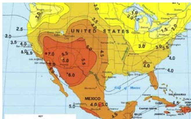
Note: Solar power output varies with geographic location and time of year. Power specifications are based on proper installation in winter sun in locations defined as "4.5" shown above. Actual power output may be higher or lower than specified. Contact GDS Corp for an analysis of your solar power requirements or for a fully custom system designed to meet your exact needs.
