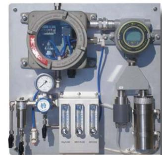
H<sub>2</sub>S and CO<sub>2</sub> Monitoring in Natural Gas Pipeline
